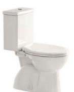
Studio Close Coupled Square Toilet Suite Soft close, quick release seat WELS 4 star, 4.5/3 ltr/flush Average flush : 3.5 ltrs S Trap : 140mm P Trap : 185mm Bottom inlet 20mm pan collar available to achieve S trap set out of 120-160mm
