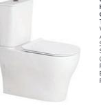
Cygnet Hygiene Rim Square Overheight Close Coupled Back to Wall Toilet Suite WELS 4 star, 4.5/3 ltr/flush Average flush: 3.5 litres Soft close seat S Trap: 140mm-260mm (180mm recommended) P Trap: 190mm Bottom and back inlet available Raised height pan
