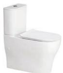
Cygnet Hygiene Rim Round Overheight Close Coupled Back to Wall Toilet Suite WELS 4 star, 4.5/3 ltr/flush Average flush: 3.5 litres Soft close seat S Trap: 140mm-260mm (180mm recommended) P Trap: 190mm Bottom and back inlet available Raised height pan
