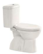
Studio Close Coupled Round Toilet Suite Soft close, quick release WELS 4 star, 4.5/3 ltr/flush S Trap : 14mm P Trap : 185mm Bottom inlet 20mm pan collar available to achieve
